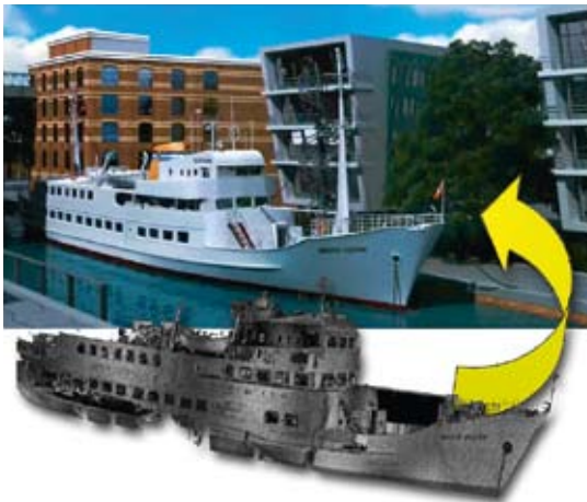
This photorealistic image was created by first modeling the boat from a point cloud as shown.*
