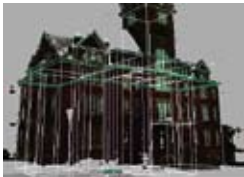
A 3D wire-frame is developed by tracing over the point cloud.
